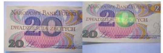
Fig 2 Variation of colour with viewing angle
